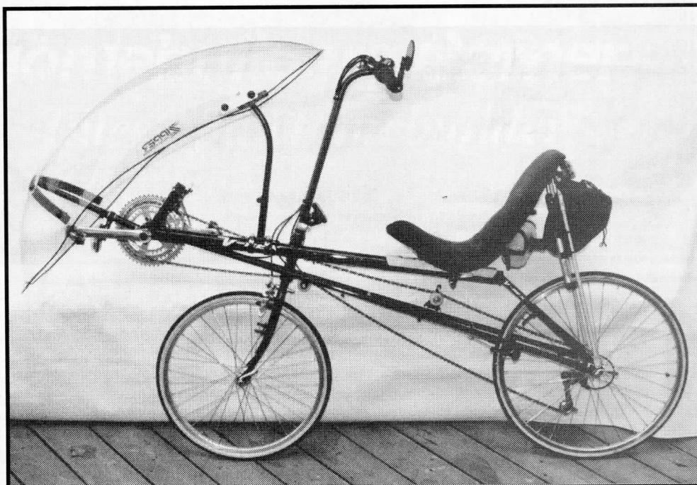
Mark Colliton's V-Rex 24/20 with 40" frame, old style seat and Zipper fairing —Photo by Mark Colliton
