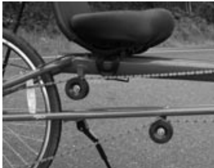
While the idlers appear wimpy in the catalog, the production versions are like robust skate wheels — smooth and quiet.
