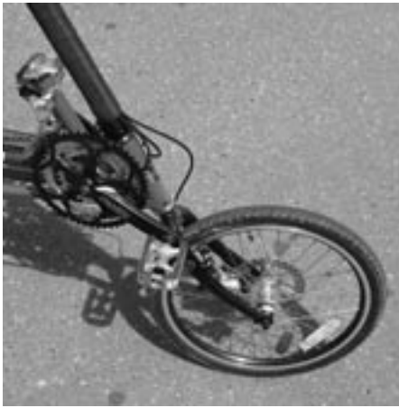
The Agio's front end clearance appears to be tight with the 165mm cranks, but there was no interference. The 1.5" tire width seems to be about right, I can't imagine this bike taking much wider tires plus fenders.
