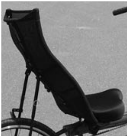
Note the upturned top of the seat back. This design doesn't work as well on LWB as it does on SWB and highracer models.
