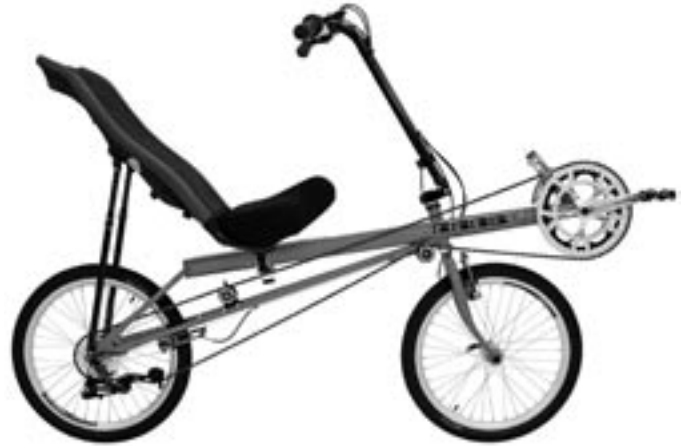
The 2006 Rocket is the most refined and affordable dual 20" recumbent made today. The upgrades include a longer wheelbase, Rad-Loc seat clamp, Flip It stem, V-brakes, full round frame tubes and a Reynolds 520 Chromoly frame all for $1174.
