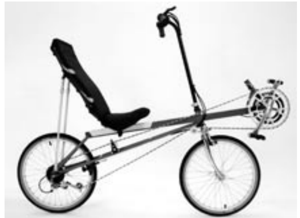
The original 1994 Rocket had a square main tube, the old style RANS seat clamp and a fixed above-seat steering. Also note long reach sidepull front brake. V-brakes solved the braking and front cable routing problems with the ingenious V-brake noodle cable mount.
