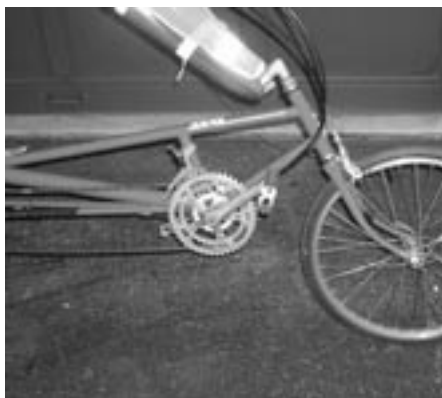
The reversed stem, an articulated riser stem would also work
