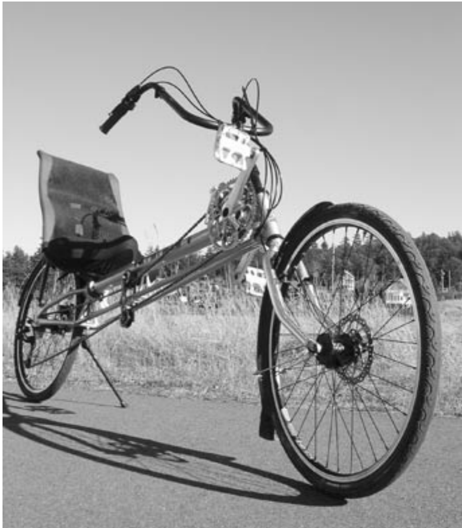
The 2006 RANS Formula 26, basically a RANS V2 Formula with head tube modification, a 26" aluminum fork and 26" wheels
