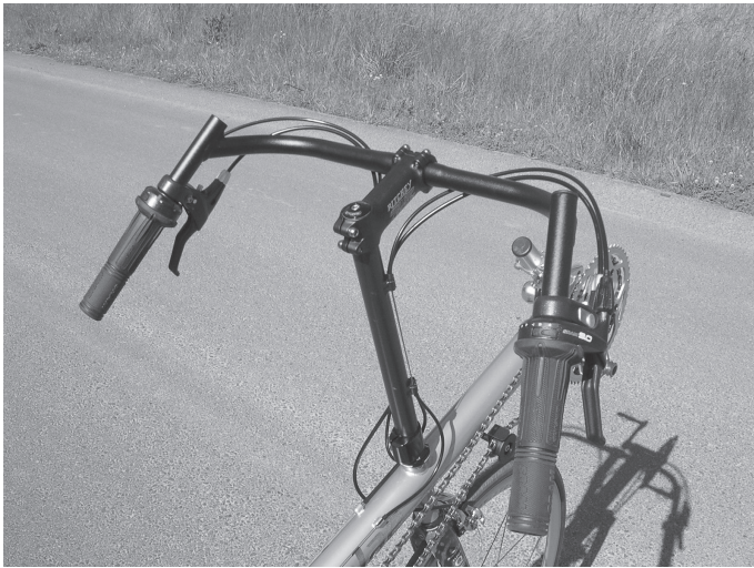
Volae's tweener style bars. A rearview mirror can be mounted on the left bar where the straight tube meets the curved section
