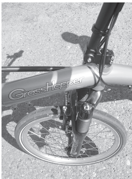
Note front suspension, OSS unit and over-size main tube
