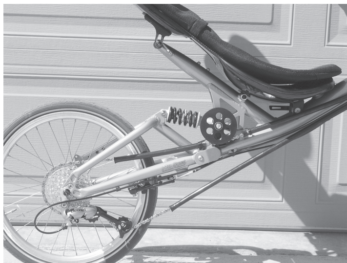
Note the sleek suspension unit and over-size chain idler along with custom chain tubes.
