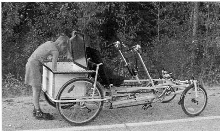
Standard 2x26 + 2x20 MicroCar with trunk
