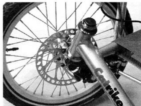
Hayes disc brakes, 16-inch front wheel, headset and aluminum frame Photo by Isaiah Charlton III
