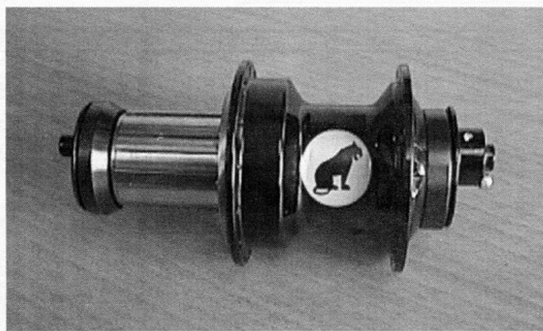
Pantour's new rear suspension hub is scarcely larger than a standard hub.
