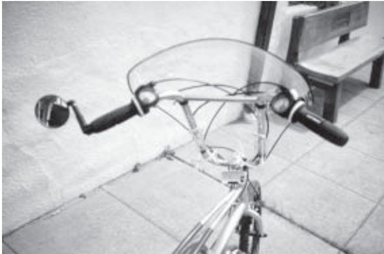
This shows the optional computer and Zipper fairing. The computer on our test bike stopped working during our test. A Super Zipper will fit this model, but you'll need Zzip Designs' T-bracket upper mounts and clamp-on lower mounts.
