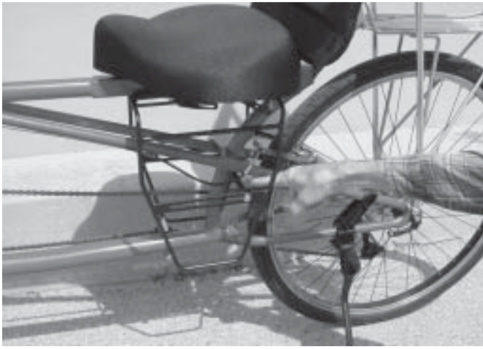
The EZ Sport underseat pannier racks. Be sure to get the EZ Sport model and not the EZ1 model, which will make for some chain slap.
