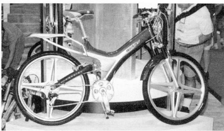
2002 Giant Prodigy "Comfort Bike" with cast aluminum wheels, disc brakes, full suspension fenders, rack and SRAM Smart bar—John Riley.
