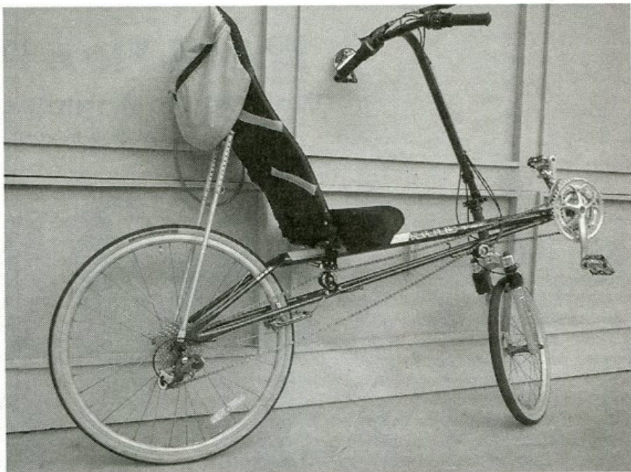
This is a stock 2000 Rans V-Rex with factory optional Ballistic front suspension fork—Bill Volk
