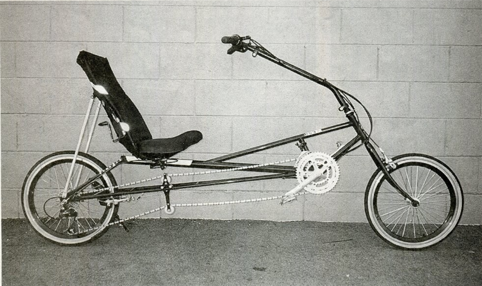
Mark Ariens' very trick Rans Stratus. Mark got a rare 24/20 model, changed the rear wheel out to a 20" and added a 700c fork.
