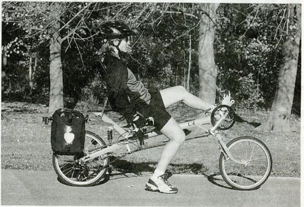
UPPER LEFT: Our C4 test bike. Note idler-free drivetrain, chain tubes, and attachment; coil/oil shock and swing arm and adjustable recline seat. We thought the seat base could use some work. It Velcros to the seat frame.
