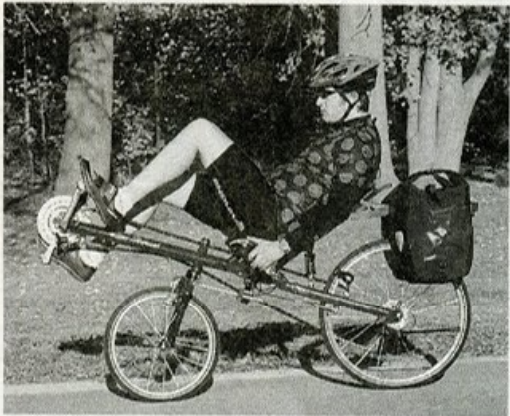
UPPER LEFT: Our C4 test bike. Note idler-free drivetrain, chain tubes, and attachment; coil/oil shock and swing arm and adjustable recline seat. We thought the seat base could use some work. It Velcros to the seat frame.
