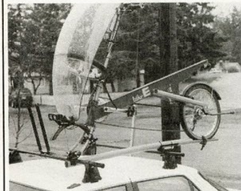
Yakima rack with custom adapter tube Photo courtesy Dan Hughes
