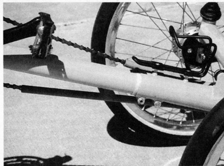
Note stock Comp Pools and plastic sleeve in boom
