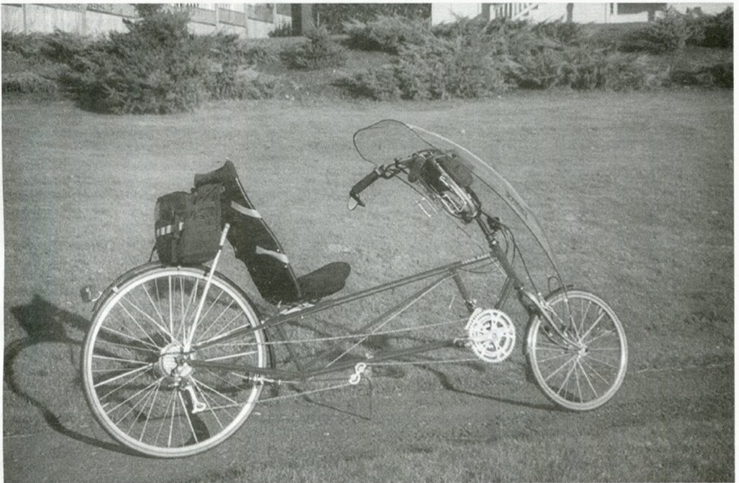
Our 1998 Easy Racer Tour Easy SS test bike with a Rans seat and Grip Shift 24-speed upgrade. The rear fender is a stock 700c with a multiple zip-tie lower mount. The seat bag is by Angletech.—RCN
