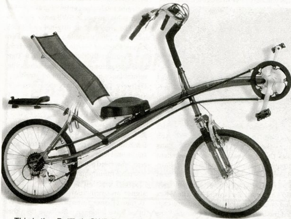
This is the Ballistic SWB Recumbent. It is very similar to German designs that we have seen. Note the high wheel interference-proof bottom bracket, dual 20" wheels, custom suspension fork and integral rack. Ballistic is primarily a suspension fork manufacturer, though they are looking for a US distributor for this, apparently mass produced-overseas, SWB recumbent.
