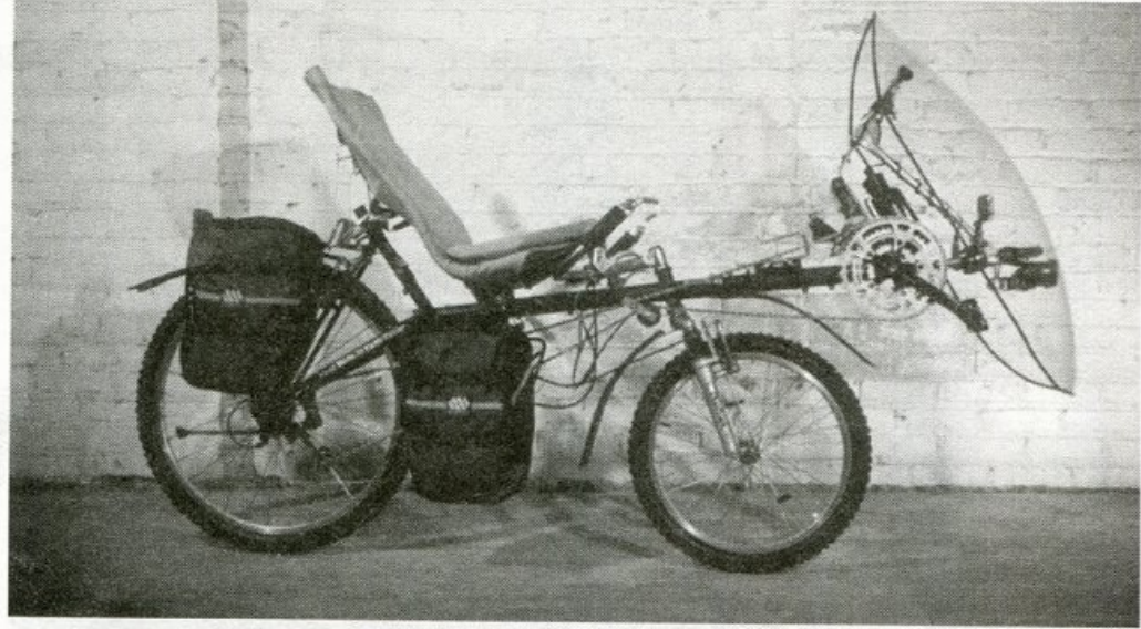
The new Earth Cycle Greenway with suspended fork, fairing and MTB options
