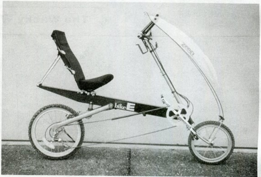
We couldn't resist...a BikeE Air Tech with a Rans seat (Tour Easy model) and 4-BikeE accessory mounts. Though completely experimental (at your own risk)—it worked great—RCN
