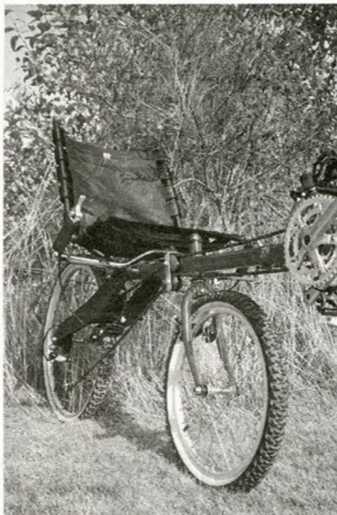
The Haluzak Traverse—a true offroad suspension recumbent
