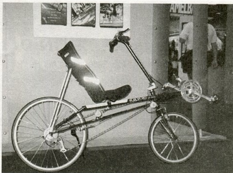
The '98 V-Rex has a 26/20 wheel combo with the 24/20 steering geometry and a 2" longer wheelbase—very dialed!
