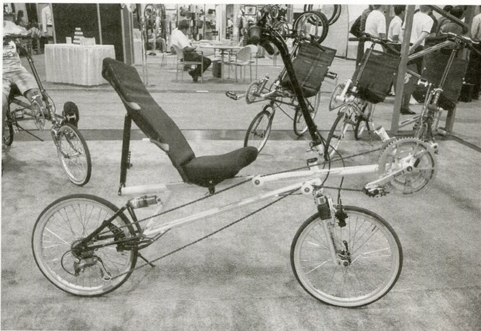
The new '98 Rans Vivo has full suspension, GripShift ESP 9.0 and Magura brakes, all for $2050. We brought the twin of the show bike home and are enjoying every moment on this very smooth, stable and excellent handling full suspension SWB.
